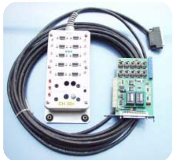
These Type-K thermocouple Converters are built into our standard 9-Pin connectors and use the miniature blade type plug. Resolution is 0.2 DegF from 32 to 1400 DegF. (or 0 to 750 C). Indicator shows any fault conditions.
