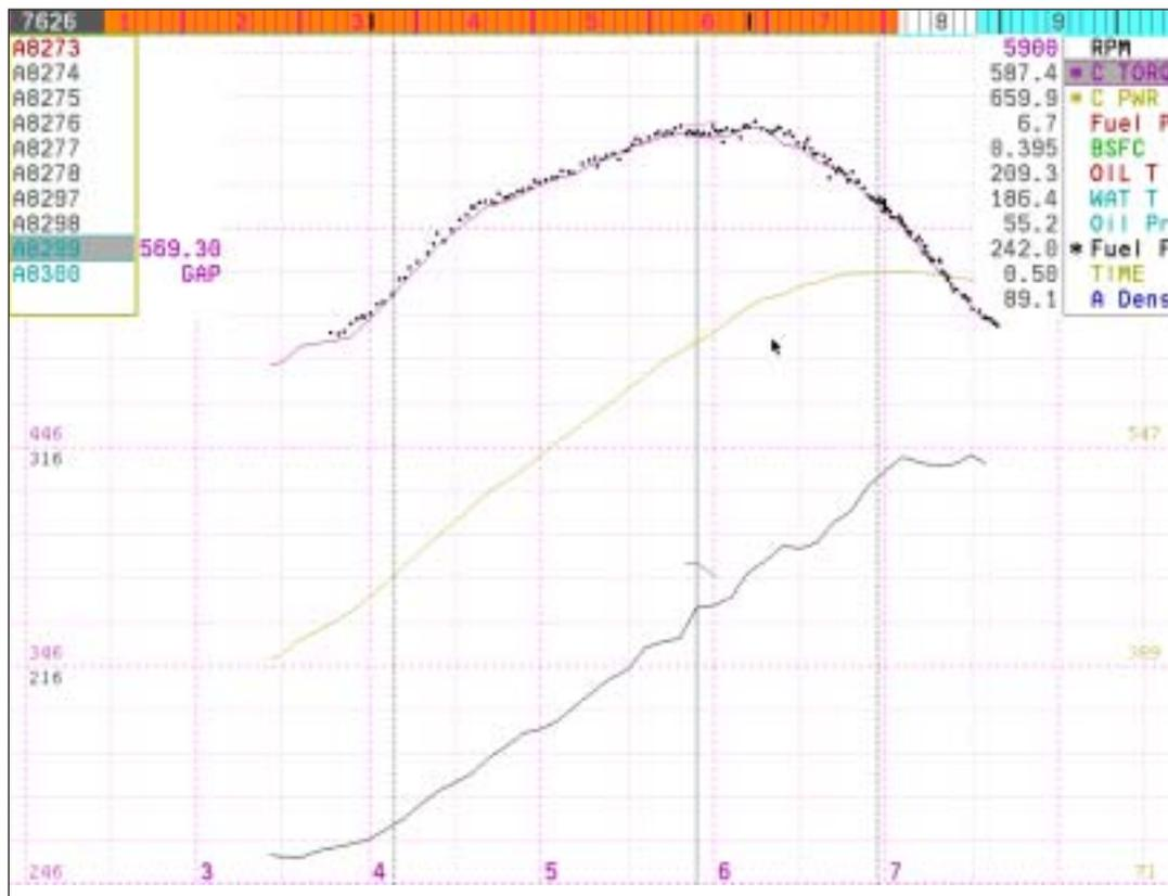
At Left is a negative image of a GrafPlot screen dump. Note the Machine-Gun dots on Torque curve for Immediate feedback on engine operation during the test run. These MGun dots can be replayed at any time just by hitting the Insert key.
